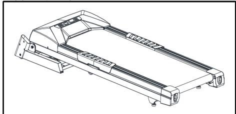
1. Remove the treadmill from the carton and position it aside on a smooth, leveled floor. The rear should be at least 3' from any wall. You must remove the plastic wrap and Styrofoam from beneath the unit before removing the Velcro belt. Tilting the unit sideways after removing the belt may cause the unit to fold and bounce upwards. This can cause serious injury.
