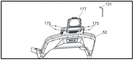
1. Insert Tablet Holder (177) into the Console Assembly (52) and use Combination M5 Allen Wrench & Phillips Head Screwdriver (131) to tighten four of Sheet Metal Screw (175).
