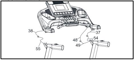
To complete this step, it is recommended that you find something to rest the console on at an appropriate height or have someone hold the console while you connect the cables.
